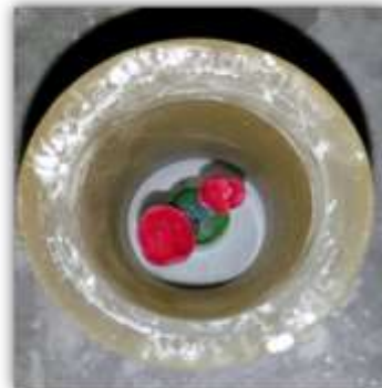
Figure no. 13. Placing of the silicone ring on the investment ring base
